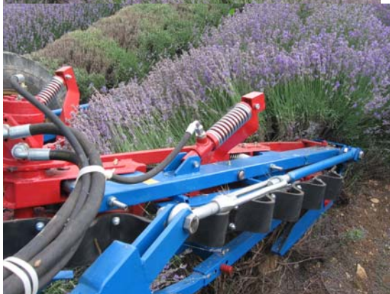
MKL 3P –Band transporter 5,5 m loading directly the attached trailer
